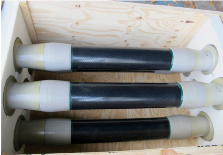
Tests of new end connectors for CF tubes
