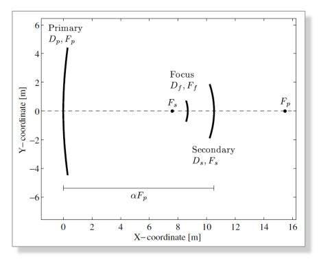
In the SC telescope, the focal plane is located in-between two aspherical mirrors, close to the secondary mirror.
